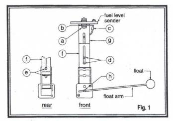
CAUTION: When installing the float arm into the sender body, make sure the float ball is to the right side when you face the unit, as shown in Fig. 1. If installed to the left, the fuel gauge will read "full" when the tank is empty.
