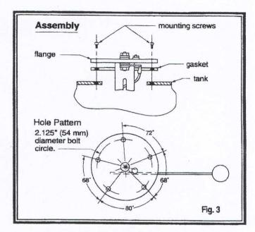
3. Insert fuel sender assembly into tank, align holes and thread in 1/2" mounting screws, through holes in sender flange and tank. Check that all screws are secure to complete assembly. AVOID OVERTIGHTENING.
